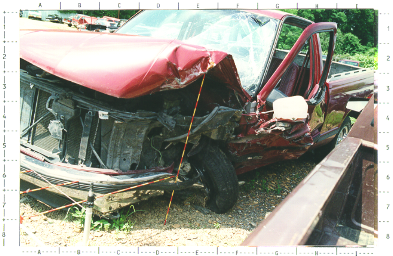
# 65 -- Front left view of damage to 1988 Chevrolet pickup; NOTE: hood damage (cells D2--E3) from contact with '91 Corsica's A-pillar
